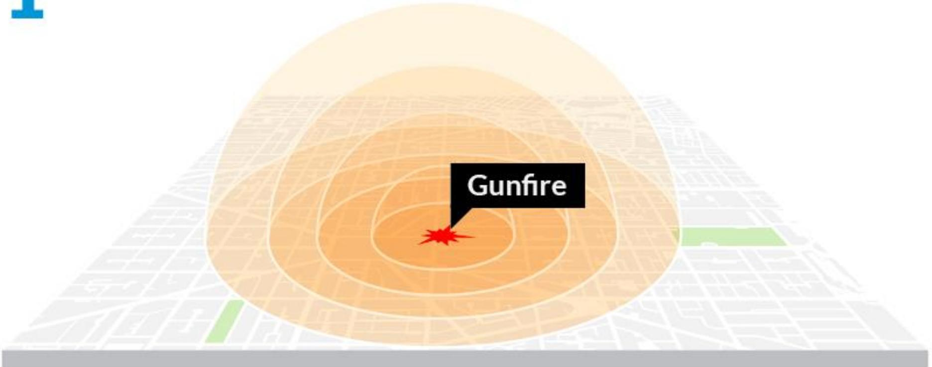
**2** Acoustic sensors throughout the city listen for the distinctive waveforms that firearms produce. When detected, individual sensors calculate the distance to the sound.
