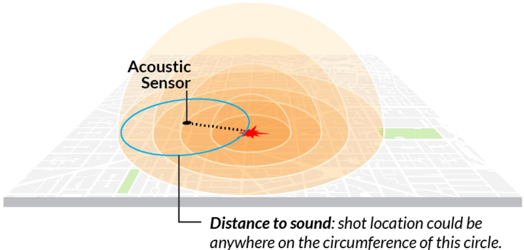
**3** Readings from multiple sensors are used to triangulate the location of the shot.
