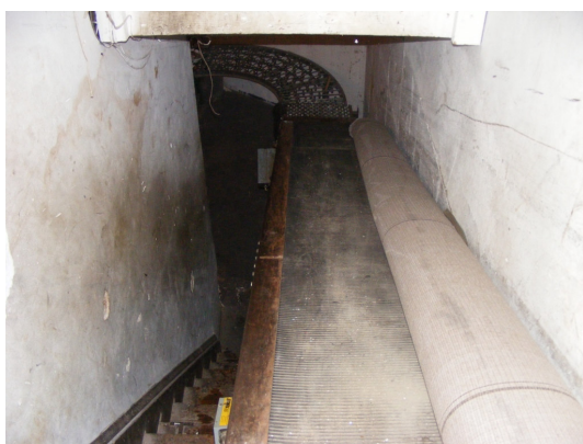
This was the conveyor belt that lead to the basement so the store manager could send very large power tools into the basement storage area.
